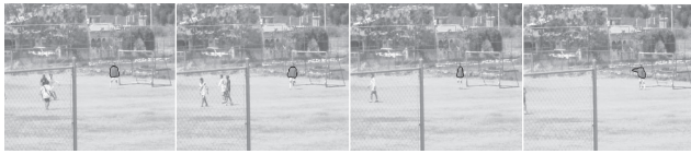
Figure 6 . Goal keeper sequence to test the fuzzy color tracking, a black line is marked to define the boundary of the object.
