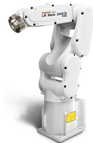
Figura 4.13: FANUC LR Mate 200iD/4SC [26].
