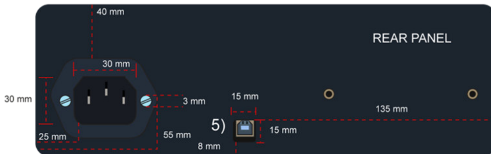
FIGURE A.7: Rear Face with the dimensions of the holes for the 4) AC connector and 3) USB B (Arduino)
