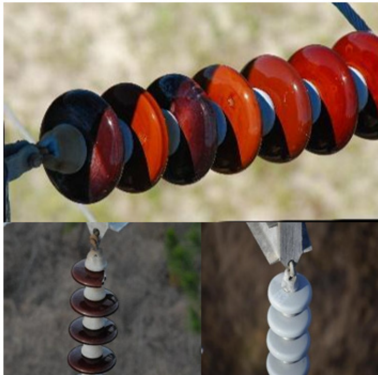
Figure A.8: Electrical insulator in good condition (top), (bottom left) broken electrical insulator, and (bottom right) insulator damaged by electrical discharge defect due to contamination.
