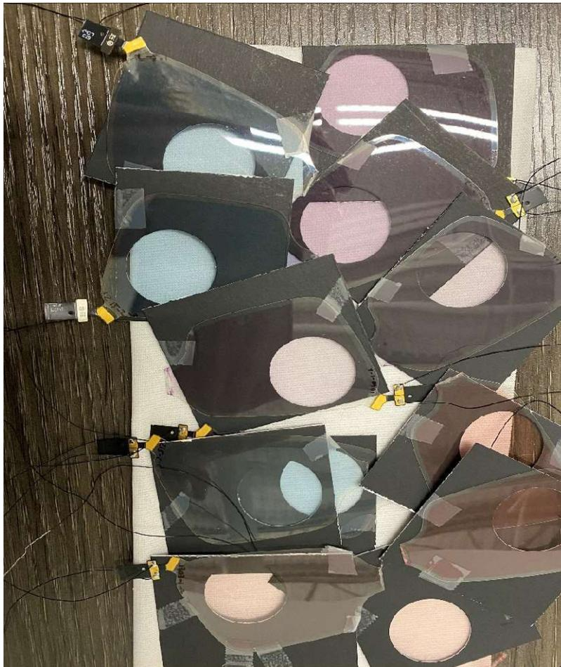
Figure 8.3.9. Example of liquid crystal cells filled with different dyes. Each cell contains a different dye mixture, resulting in variations in color and light absorption. The selection of dyes influences the optical properties of the cells, which can be tailored for specific applications.
