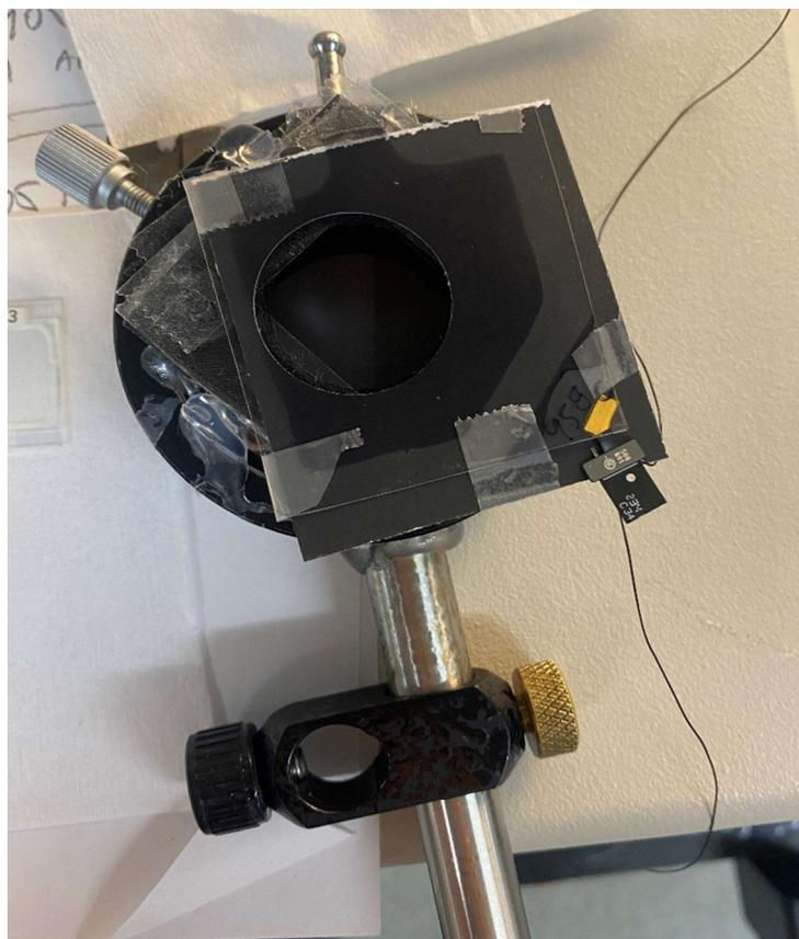
Figure 8.3.6. Placement of the cell in a holder for optical characterization
