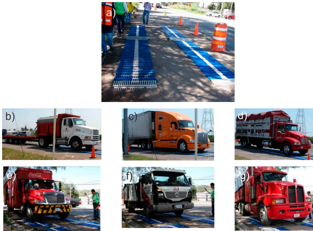
Figure 3. Implementation and execution of surveys. (a) Placement of portable PAT. (b–g) Some measured trucks. Pictures are either by the authors and/or by the IMT reports hired by UG [22,23].
