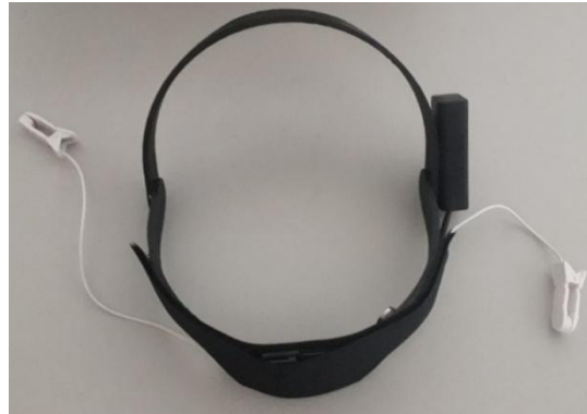
Figure 19. Headband for recording EEG potentials.
