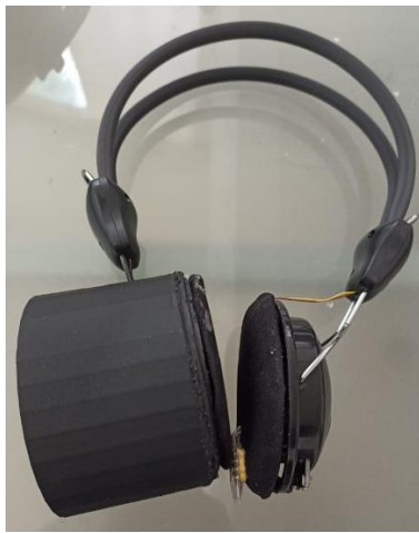
Figure 6. MAX30102 sensor attached to an adjustable headband that allows the sensor to remain in position.
