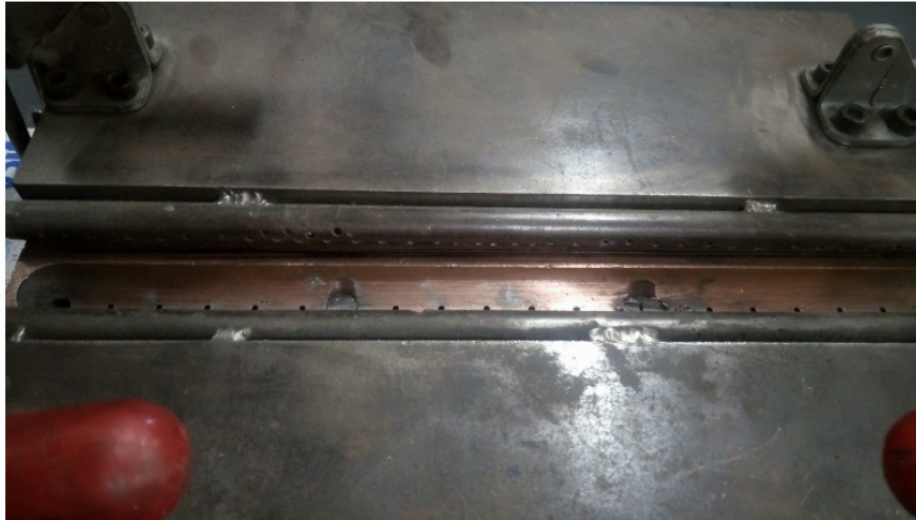
Figure 1. Protection chamber used during welding the FSS of this research. Source: Author's own elaboration.
