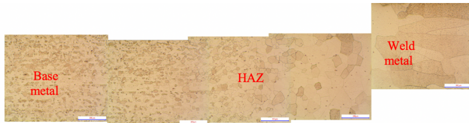
Figure 5. Microstructure of sample 3 at 100X. Source: Author's own elaboration.
