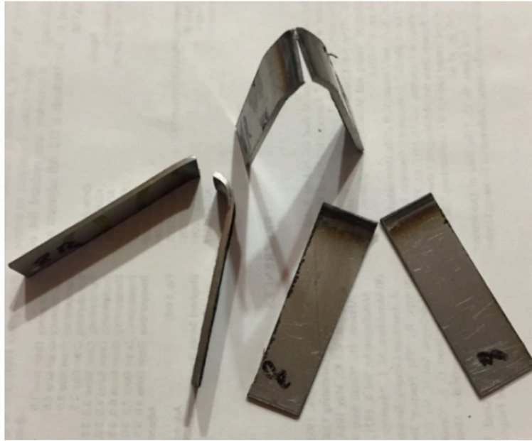
Figure 6. Bend test specimens of sample 1 after being tested. Source: Author's own elaboration.
