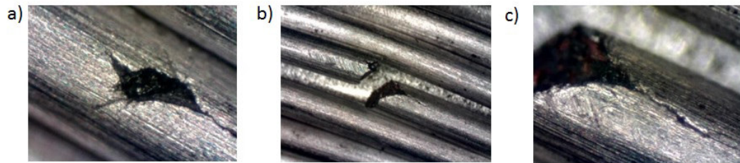
Figure 2.35: Dissection of cable sample 3. The tear shown occurs after the outer sheath welding process and the bending tests, most likely due to the strain at the bend. Figure at left shows the breaking point of the strand. The image at right shows a close-up image of the tear.
