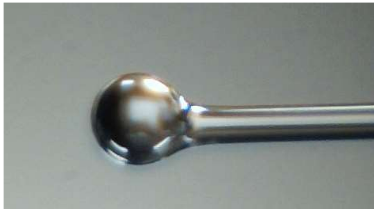
Figure 1.1: Result of the optical fiber and the spherical MR fabricated. In this case, a 335 \mu\text{m} sphere is obtained from a 125 \mu\text{m} in diameter optical fiber.
