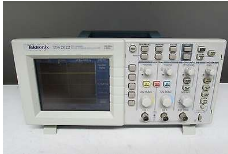
Figure 3.11: Two channel 1 GS/s sample rate oscilloscope used to monitor the FG and the Photodiode signals, capable of detecting resonances that takes 60 \mu\text{s} to occur.
