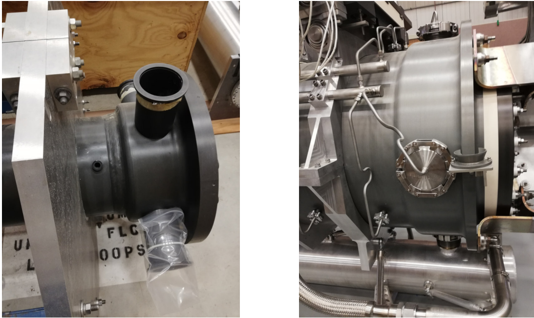
Figure 7.1. Left: picture of horn 1 outer conductor of NuMI beam, only 3 visible drain holes on the image. Right: drain holes on horn 2 of NuMI beam, only the bottom drain hole is used to drain water and gas, a pump is used to drain to a water tank to process and reuse the fluids, the 3 remaining drain holes are used as input of water and gas (Argon for NuMI).
