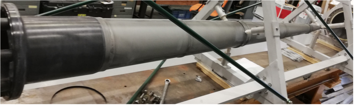
Figure 6.3. Current Equalizer Section in horn 1 (black section on the left).
