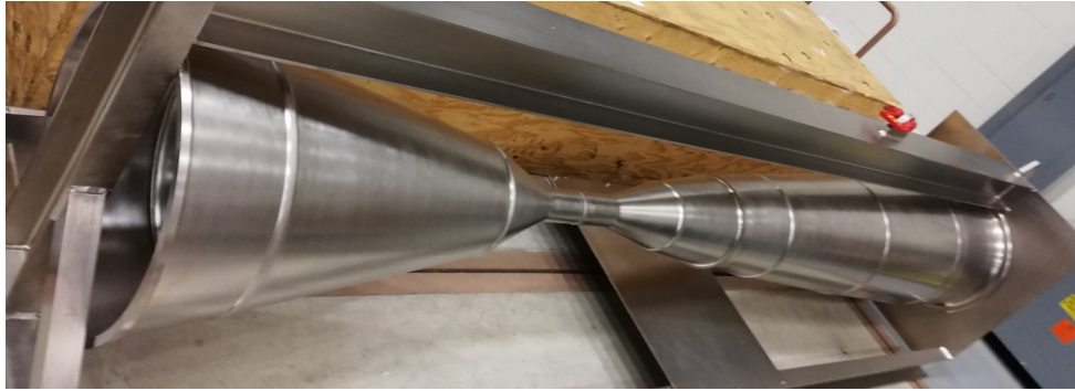
Figure 3.10. Picture of horn 2 inner conductor.
