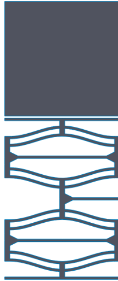
Figure 4.11. 2D half-structure with falling block model .
