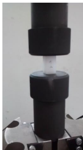
Figure 2.17. Load appliance on specimen during compression test.
