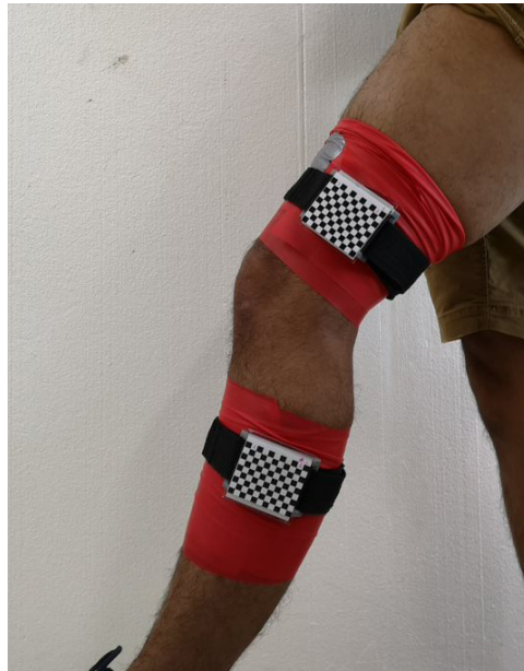
Figure 5.4: Final tracking system on the left leg of a volunteer.
