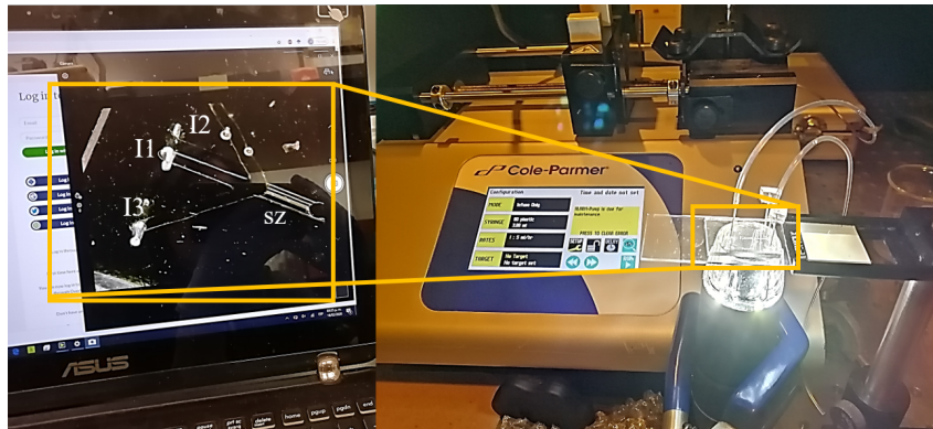
FIGURE 4.3: Experimental test of fluid leakage. It is possible observe a microcamera, the employed micropump, serynger and the system to visualize the device. in the inset are shown the sorting zone (SZ) inlets I1, I2 and I3.
