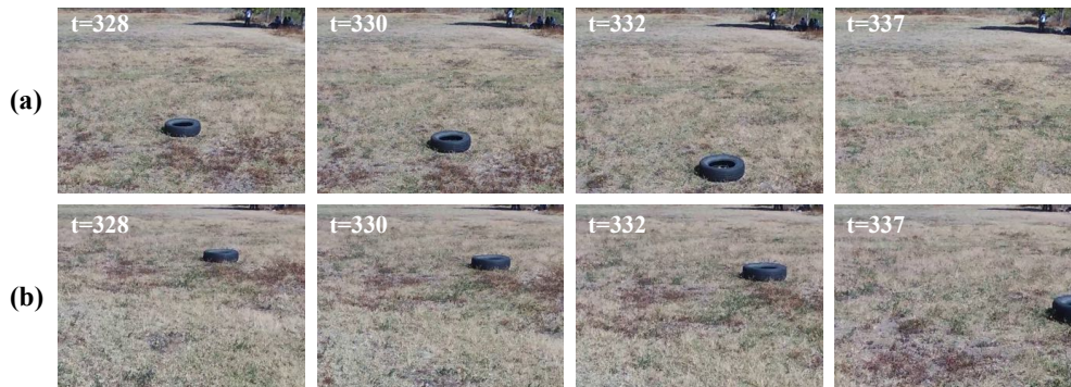
Figure 3.18: Failure cases in the evolved GWR detector on D-4 dataset, (a) sample image frames in the exploration phase, and (b) false novelty indications in the inspection phase. In the exploration phase, the UAV explores the environment O-3. Then, it should detect the person as the novelty in the environment O-4. In the inspection phase, due to changes in perspective in the frames induced by the UAV flight, some false novelty detections are presented because the information of the frame encoding is too different to the learned model.
