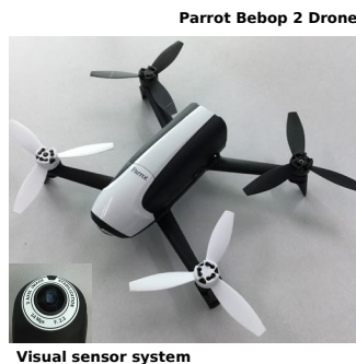
Figure 3.5: Parrot Bebop 2 Drone with a 14 Mpx flight camera. In the bottom-left corner, we show its visual sensor system.
