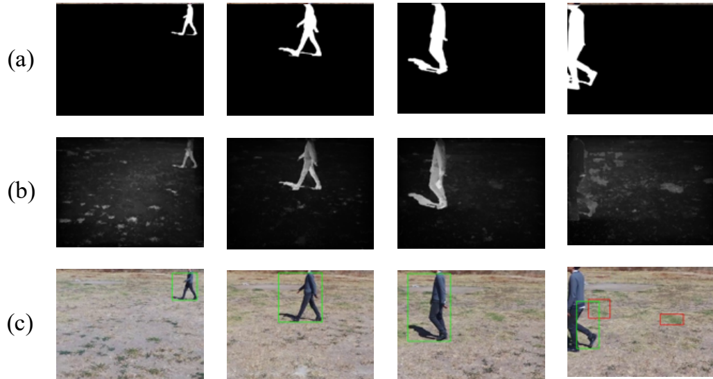
Figure 5.1: Novelty localization based on saliency detection. (a) Reference novelty indication, (b) Saliency detection with the Minimum Directional Contrast algorithm, and (c) Patches detected as novel objects by the grow-when-required network (green bounding boxes).
