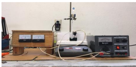
IMAGE 10: Electrodeposition of Copper with ammeter, Voltmeter.
