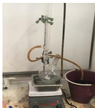
IMAGE 3. System to carry out the leaching in a 500 mL 3-necked flask, at a water bath and at reflux with cooling water.
