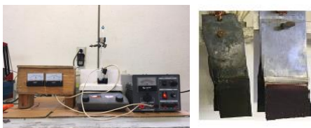
IMAGE 13: Equipment used for electroposition of copper.
