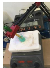
IMAGE 7. Add NaOH in flask with mechanical agitation of 600 rpm. In order to pH 3.
