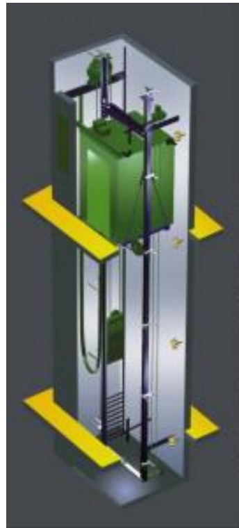
51. mecanismo de Ascensor (ascensorssales,2020 https://n9.cl/aic )
