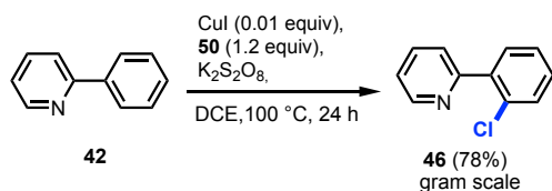
Scheme 17. Copper-catalyzed ortho -chlorination of aryl pyridines. (A higher resolution / colour version of this figure is available in the electronic copy of the article).
