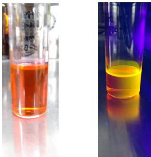
Figure 46. Left: solution of compound 275 in DCM under normal light. Right: solution of compound 275 in DCM under UV light at 365 nm.
