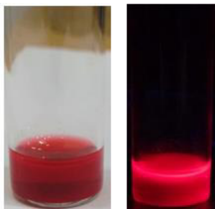
Figure 36. Left: Compound 193 under normal light. Right: Compound 193 under UV light at 365 nm showing red fluorescence.
