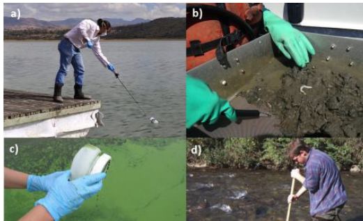
Figure 10. Sampling approaches in rivers and reservoirs for a) water, b) sediments, c) algae, and d) macroinvertebrates
