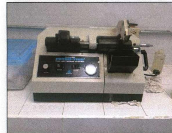
**Figura 6.** PETRO-THIN thin sectioning system
